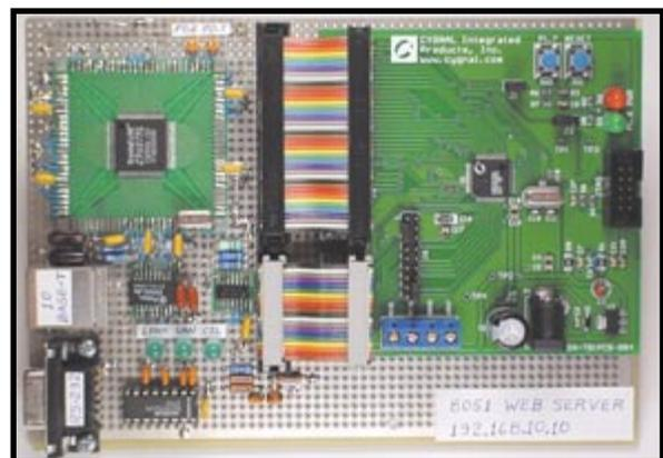
Photo 1—The Cygnal C8051F005TB sits atop my breadboard at the upper-right. The top ribbon cable connects the 8051 CPU to the CS8900A Ethernet controller while the lower ribbon cable carries analog signals.
