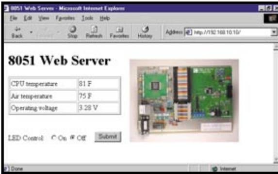
**Photo 2**—Seeing is believing! The web page and image served by the 8051 can be seen in the browser window. The on/off buttons control the state of an LED on the breadboard.
